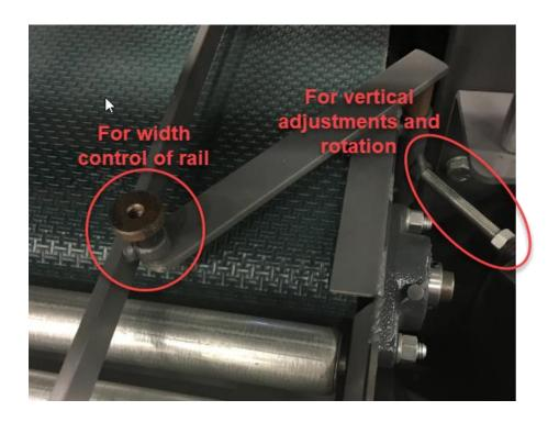
When adjusting the tension on the belt, tighten it just enough to move with the rollers. Belt tension **does not** need to be tight enough to stretch the belt.
