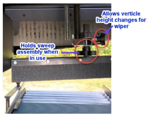
13. The rotary brush should brush the top of the container slightly. Lower the brush to remove additional material from the container.
